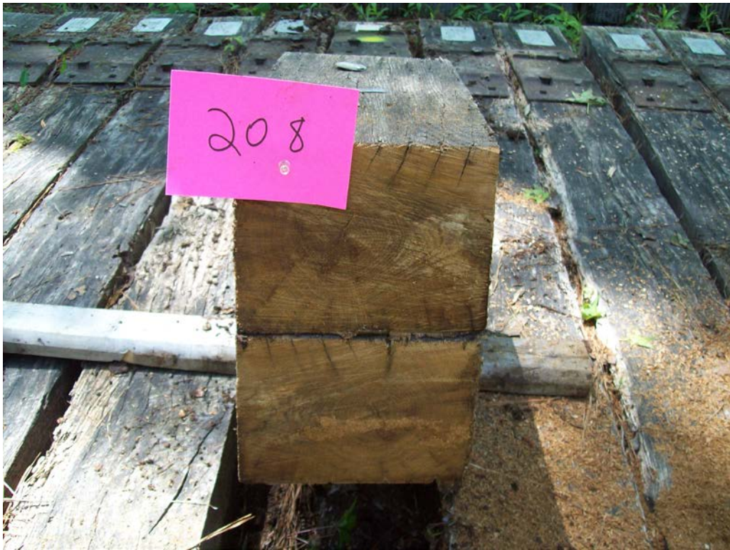
Figure 42 - Tie #208 (Nisus/white oak/borate) with decay on bottom.
