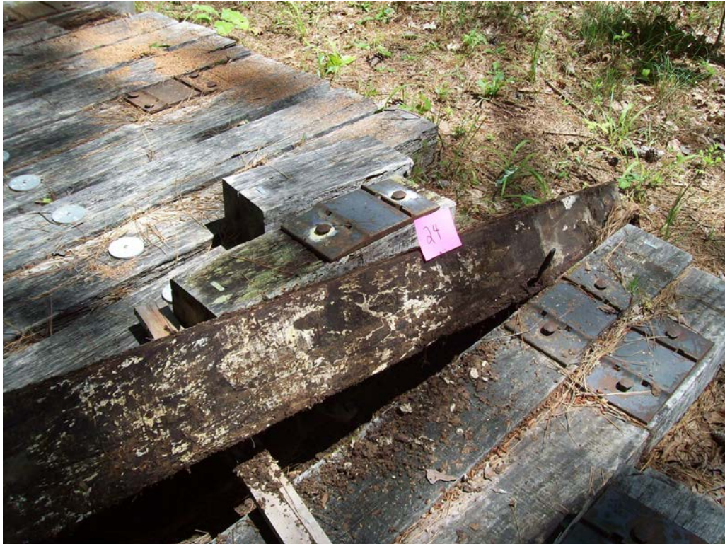
Figure 5 – Tie #24 (Turada) with light decay on bottom.
