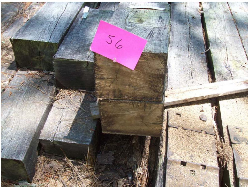
Figure 10 - Tie #56 (Boatright/white oak/borate/creosote to refusal).
