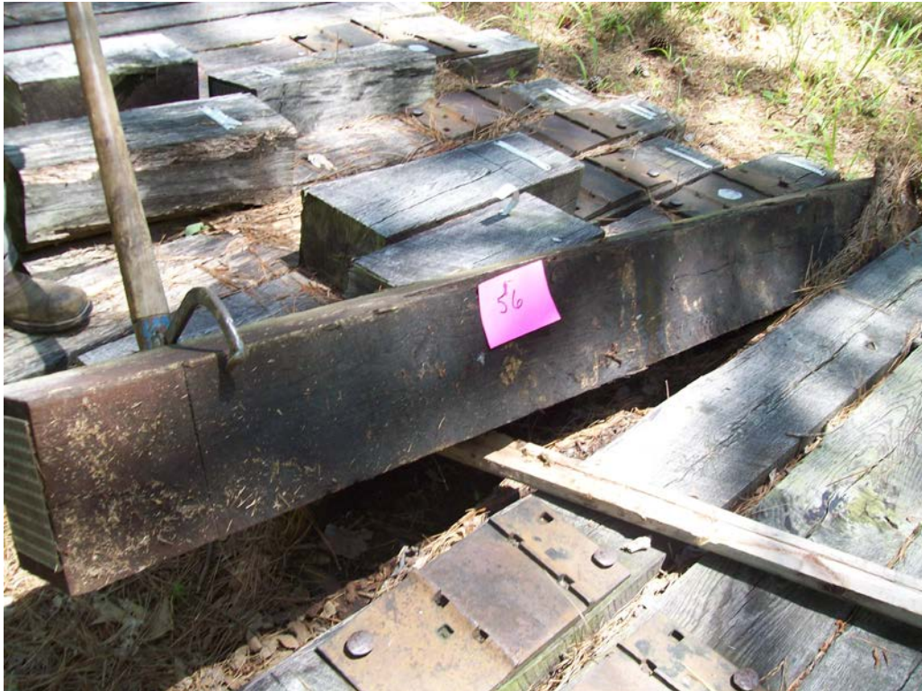
Figure 9 - Tie #56 (Boatright/white oak/borate/creosote to refusal).
