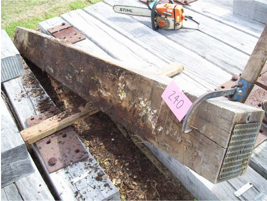
Figure 45 - Tie #240 (Merichem/white oak/borate/CuNap) with slight decay.
