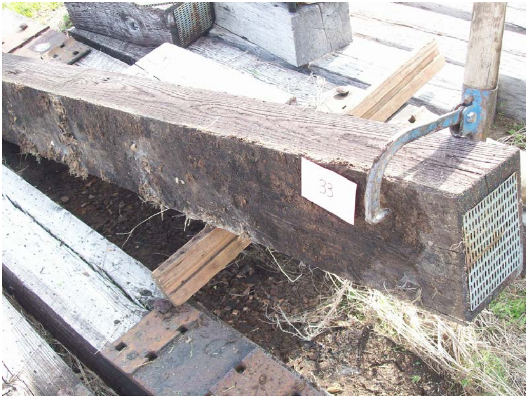
Figure 7 – Tie #33 (Boatright/red oak/creosote 5pcf).
