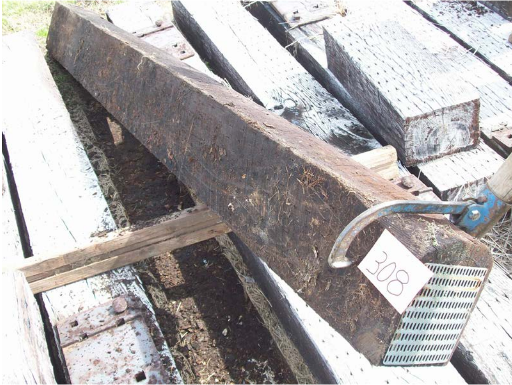
Figure 523 - Tie #308 (Koppers/white oak/creosote petroleum solution).
