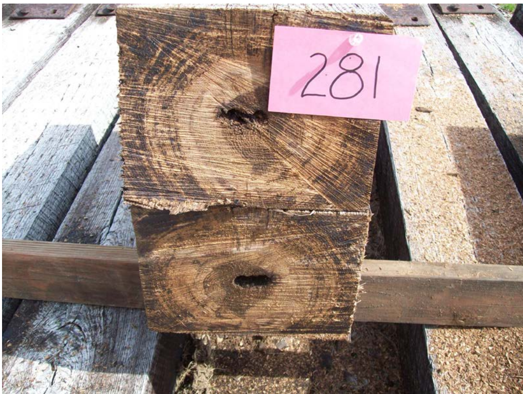
Figure 490 - Tie #281 (KMG/red oak) with heart decay.
