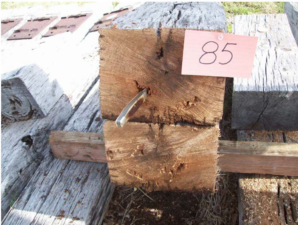
Figure 18 - Tie #85 (Lonza/red oak) decay evident in cross-section.
