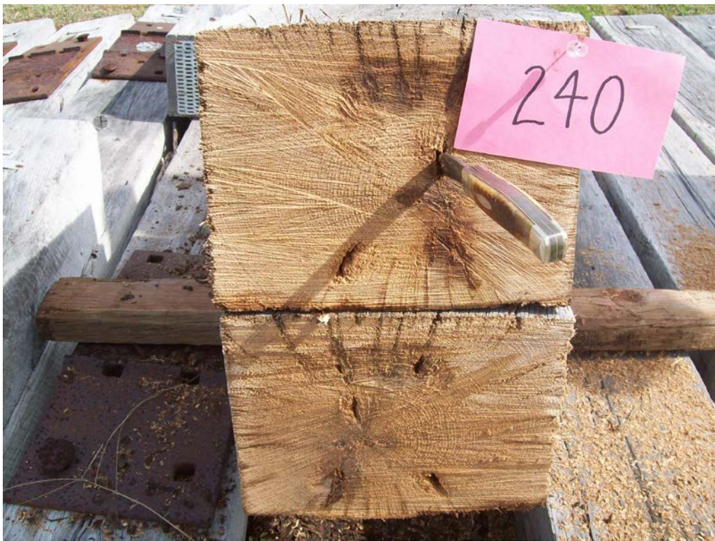
Figure 46 - Tie #240 (Merichem/white oak/borate/CuNap) with internal decay.
