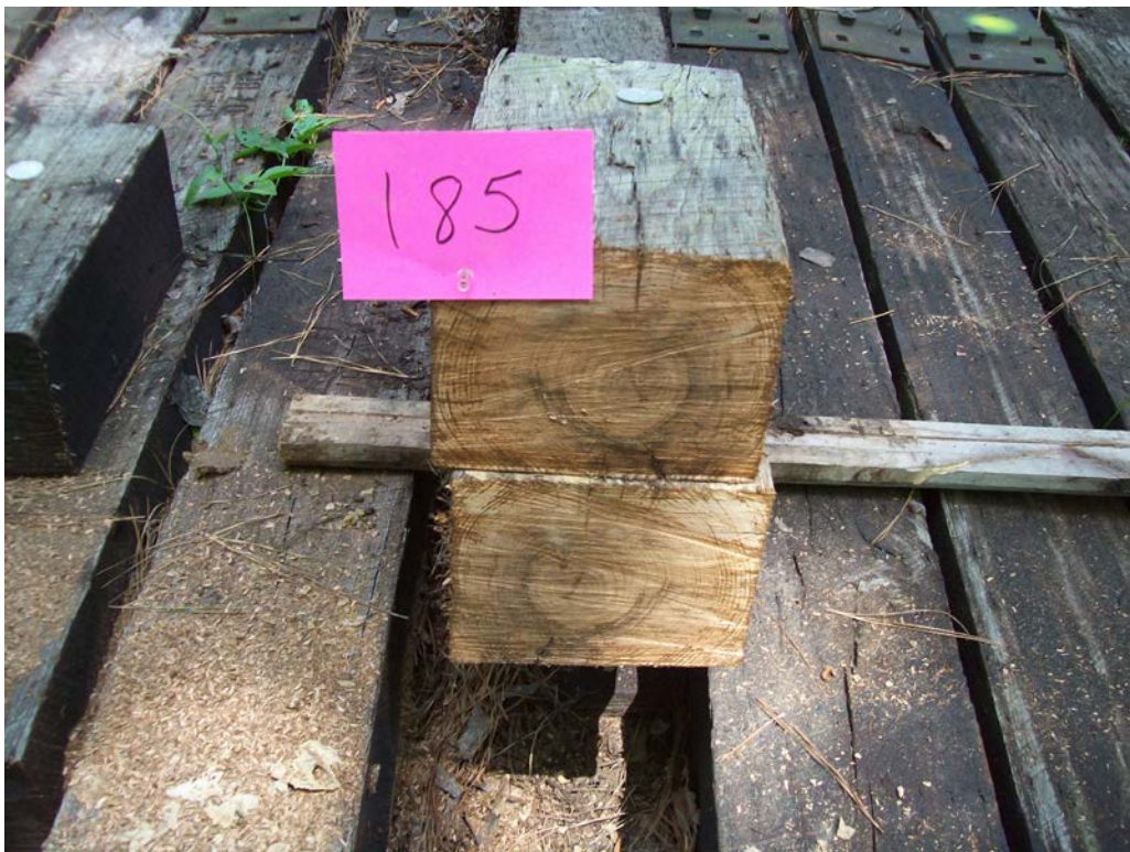
Figure 36 - Tie #185 (Nisus/red oak/borate/oil B).
