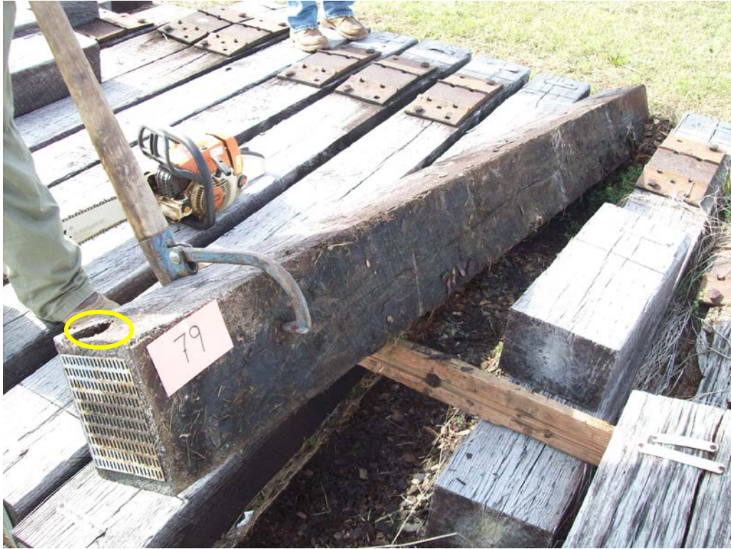
Figure 15 - Tie #79 (Boatright/red oak/borate-creosote 7pcf) large knot on side.
