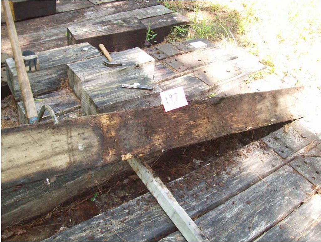
Figure 39 - Tie #197 (Nisus/red oak/borate) decay on bottom.
