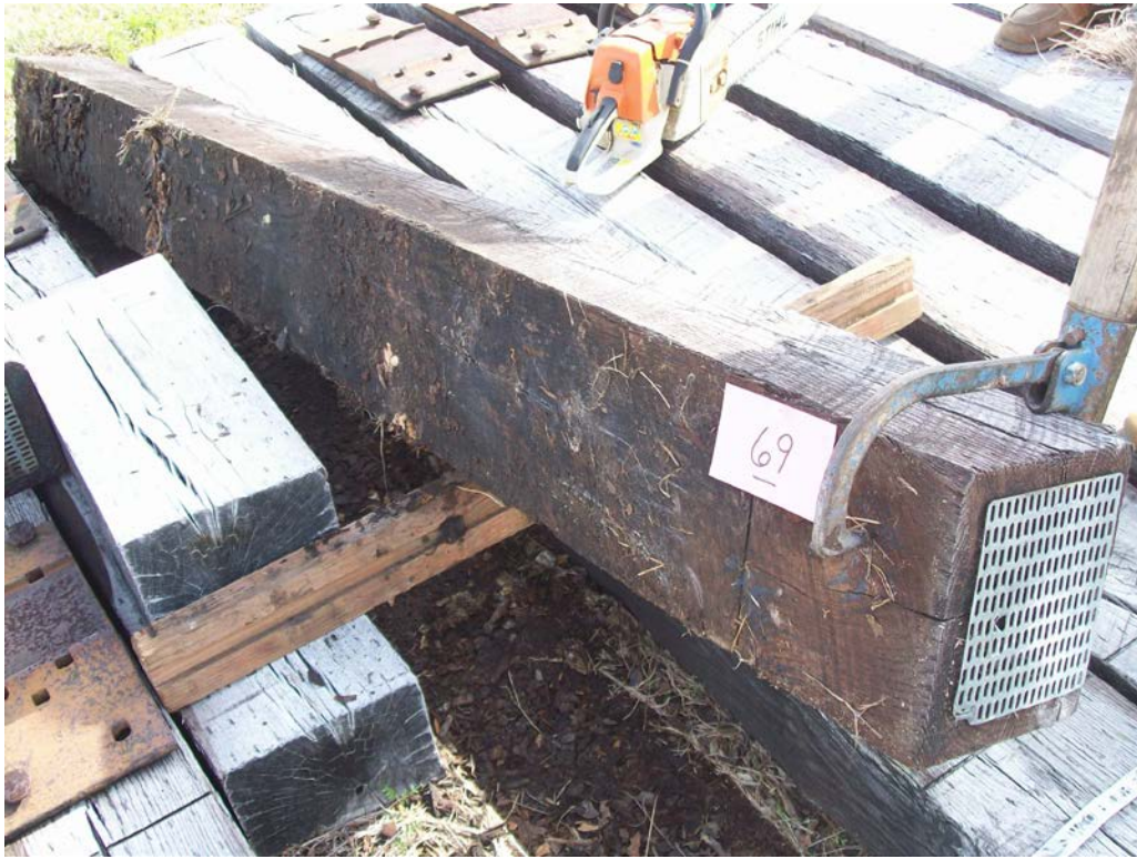
Figure 13 - Tie #69 (Boatright/white oak/borate-creosote to refusal).
